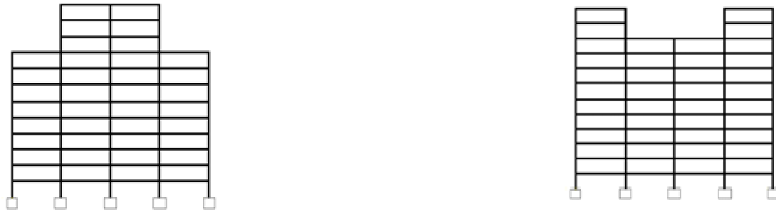
Figure 5(a-e)Types of 12s4b bare frame regular and irregular buildings (a) 12s4b RB(b) 12s4b IBD1 (c) 12s4b IBD2 (d) 12s4b IBD3 (e) 12s4b IBD4
