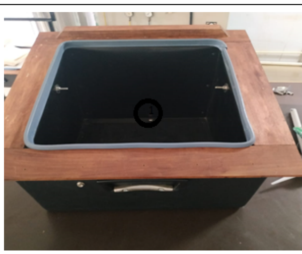
Figure 2 . The interior part of the cooking chamber painted black.
