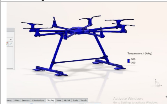
Fig. 3 Temperature contour of drone of forward motion
